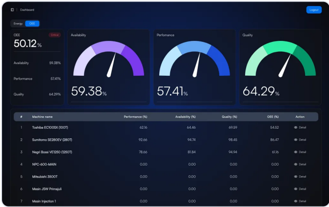
OEE per machine and per shift, computed from machine signals.
